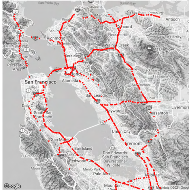
Figure A12: This figure plots traffic sensors from the Caltrans Performance Measurement System (PeMS). Each sensor reports hourly vehicle count and speed data that are converted to traffic density (vehicles/lane/mile) using the fundamental diagram of traffic flow. These traffic density readings are then used to assign congestion externalities to vehicle trips based on route and time of day, as described in sections 5 and 8.
